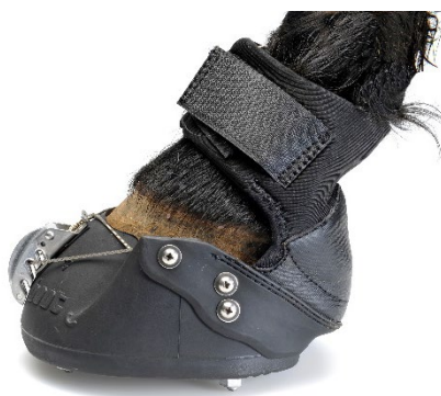
Figure 63 Hoof boot made of polyurethane. It is used to replace or supplement shoeing, as well as to protect a hoof (mainly the sole) that is injured, weakened or undergoing treatment (Source: Swiss Army (2021) - documentation - military farriery 64.010 f. With the kind permission of Colonel S. Montavon, Swiss Army Veterinary Service)
